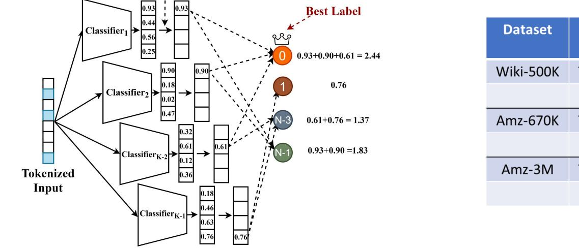
Schematic diagram for Inference. We first get **K** probability vectors of **B** dimensions each. Then we only retain the **top-m** buckets after sparsification (**m**=1 in above figure. For our experiments, **m** varies among 50 and 100). We accumulate the candidate labels based on inverted-index for these top-buckets and aggregate their scores and identify the best labels
